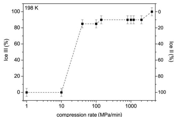
FIG. 3. The effect of variation of compression rate on the fraction of ice III in the ice II/ice III mixture produced by compressing hexagonal ice isothermally at 198 K. The error bars indicate the reliability of the POWDER CELL (Ref. 44) fit of ice II and ice III patterns to the observed powder x-ray diffractograms.
