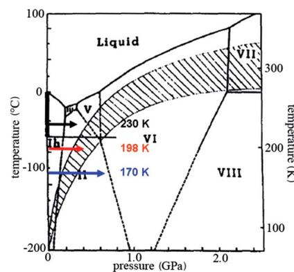
FIG. 1. (Color online) Water's phase diagram of stable phases. The shaded area indicates the approximate pressure and temperature conditions in the interior of the icy satellites of outer planets. The arrows indicate the paths taken for the uniaxial compression experiments of hexagonal ice. The figure was adapted from Leliwa-Kopystynski (Ref. 10).
