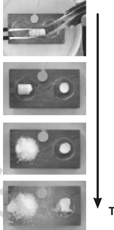
**Figure 7.** Amorphous ice sample (1.5 mL) made by decompression of VHDA (see Section VII) at 140K to 0.07 GPa with a rate of  $13 \text{ MPa min}^{-1}$  and then quench-recovered to 77K and 1 bar (top image). After removal from the piston cylinder apparatus, the sample easily broke into two pieces; the two separated pieces were placed on a copper block kept at 77K (second from top). The bottom two images show the two pieces in the course of heating to 250K at 1 bar.
