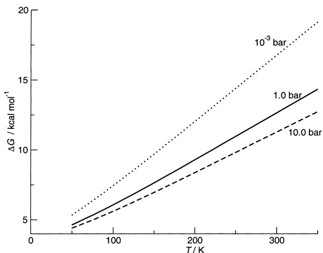
Figure 1. Free-energy change for the formation of  $\text{H}_2\text{SO}_3$  according to the reaction  $\text{SO}_2 + \text{H}_2\text{O} \rightarrow \text{H}_2\text{SO}_3$ . Three different pressures were investigated, namely 0.001, 1.0 (standard state), and 10.0 bar. The energies were determined at the CCSD(T)/aug-cc-pVTZ//MP2/aug-cc-pVTZ level of theory, and zero point corrections were obtained with MP2/aug-cc-pVTZ.
