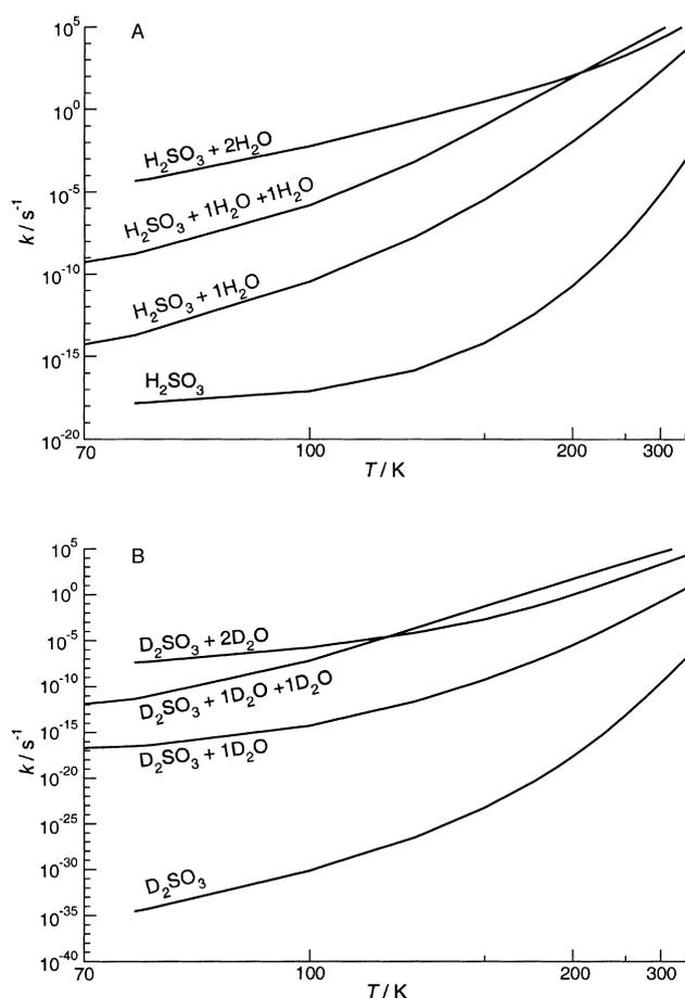
Figure 3. Reaction rates of sulfurous acid decomposition, as a function of temperature, as catalyzed with no, one, or two water molecules. A) reaction rate constants with the  $^1\text{H}$  isotope, B) reaction rates for the deuterium ( $^2\text{H}$ ) isotopes. In both cases quantum-mechanical tunneling is important. The contribution of tunneling is lower for the deuterium-substituted reaction channels, thus the cross-over between  $n = 2$  and  $n = 1+1$  occurs at lower temperatures.
